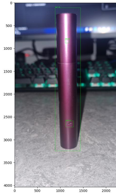
Figure 32. After 10,000 training steps, the model was able to detect the object and defects.
