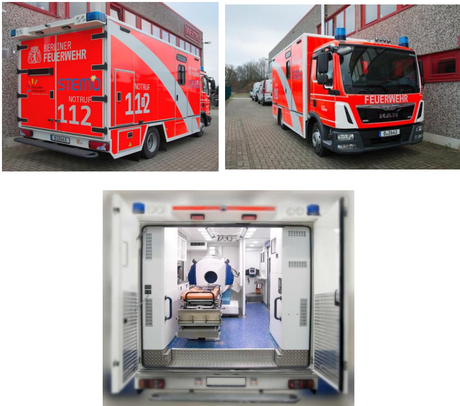
Figure 1.3. An MSU in Berlin, Germany, and its side, including the CT scanner [15]. Used with permission, copyright MEYTEC GmbH.
