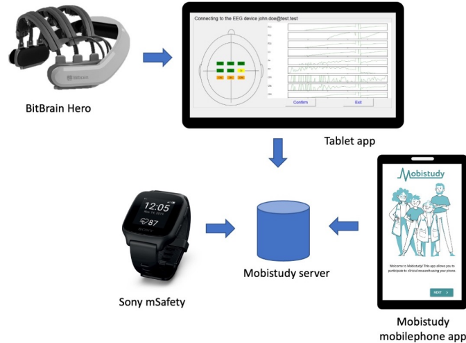
Fig. 1. IoT-base system architecture including sensors (Sony mSafety and BitBrain Hero), user applications (Mobistudy app and tablet app) and server.
