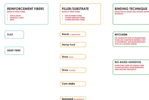
Fig. 4. The classification of the selected materials (natural fibres and fillers/substrates) and the targeted binding techniques.
