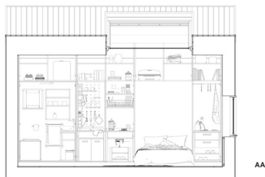
Fig. 2. Section AA showing the detailed design for all eco-cycle details in the bathroom and kitchen integrated with furniture.
