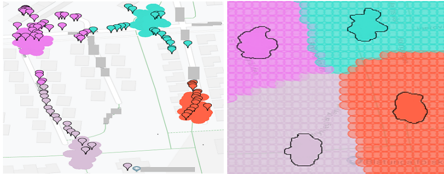
Fig. 2. Location feature space, markers represent predictions, blobs represent teaching data and areas are classification boundaries.
